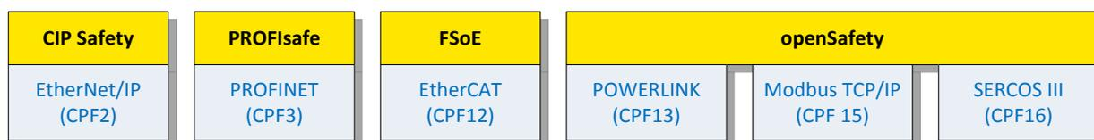
Figure 3: Safety over Industrial Ethernet Protocols
