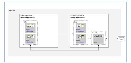
The concept is discussed with the TÜV Rheinland for safety systems up to IEC 61508 - SIL3 and is depicted in following block diagram. SAFEFLEX — FSDK is supporting now fieldbus communication with a safety protocol. The first supported fieldbus is the Ethernet POWERLINK from our partners EPSG and Softing. openSAFETY from EPSG is used as safety protocol.
